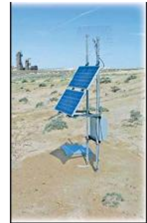
Microseismic Downhole Sensors and Surface Completion with Solar Power (ESG)
